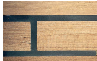
Fig. 29 New teak deck
