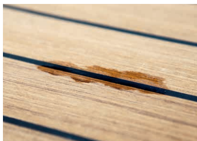
Fig. 32 Discolouration of the wood is a tell-tale sign of a failed or damaged joint in this teak deck
