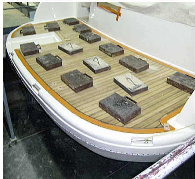
Fig. 27 Holding in place with weights
